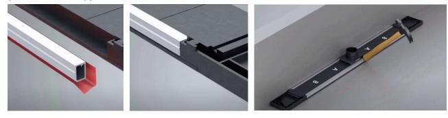
**Drill and Countersink for Rail Attachment Screws:** Use the Drill Guide, Countersink Guide, and Drill Bit to make six countersunk holes through the Drain Body and Rails. Screws should be roughly placed at each end and center of both Rails. Do not over-tighten the Screws.
