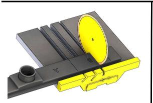
Final Cut of the Drain Body: Cuts can be made with a variety of tools, however, make sure cuts made to the Drain Body are <u>NEAT and SQUARE.</u>
