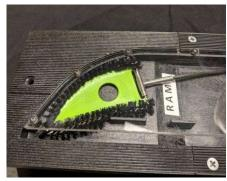
3. Holding the D-shaped Brush with your finger, lower the Brush into the Access Opening with the straight side parallel to the Drain Channel. Push the Brush forward into the Main Channel and pull back and forth several times to clean. If possible, avoid rubbing the Brush shaft on the lower perimeter of the Access Cover Frame.
